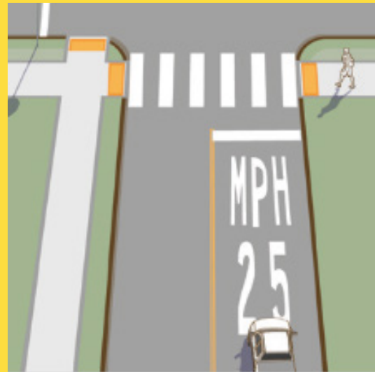
Speed Limit Pavement Marking*
