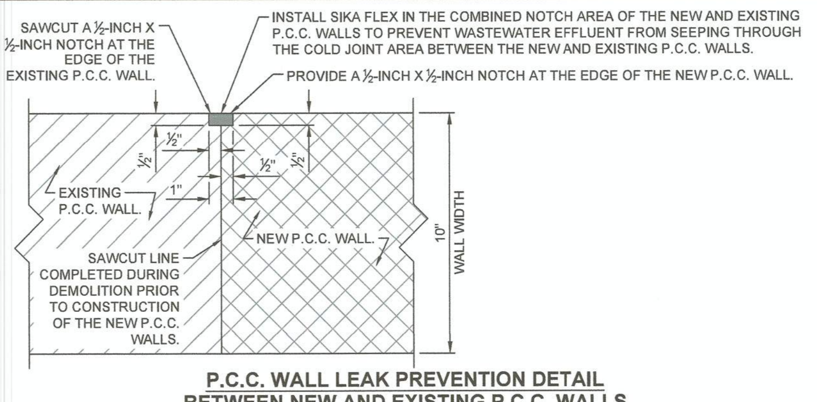
DEMOLITION AND REPLACEMENT OF P.C.C. CHLORINATION / DECHLORINATION WALL SECTIONS SCALE 1" = 1'
