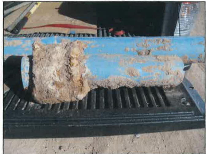
Existing 4-inch force main pipe removed from the trench.
