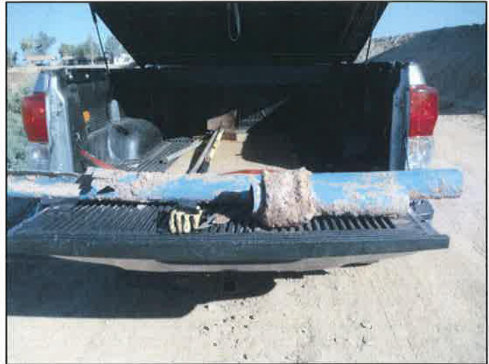
Existing 4-inch force main pipe removed from the trench. Note the splintered section on the left, repair coupling in the middle, and the barely visible chip and crack in the spigot end of the shorter section on the right.
